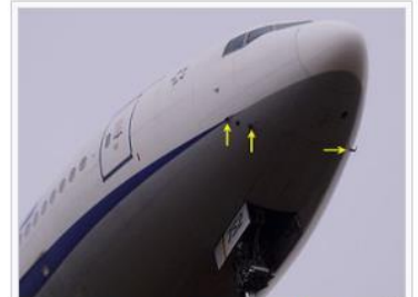
Location of pitot tubes on a Boeing 777
